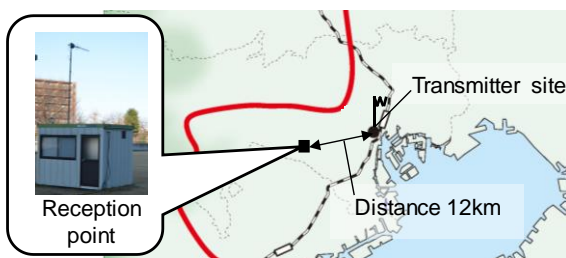
Figure 10 – The reception point for the 4K/8K video transmission experiment
