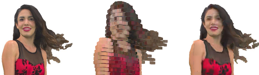
Figure 4 – Original, anchor (8), and V-PCC decoded point cloud at 3.5 MBit/s.
