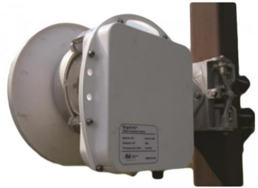
Figure 14, 60GHz Wireless Uncompressed HD SDI Link
