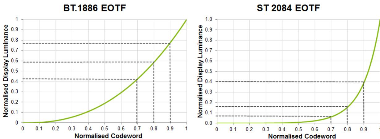
Figure 1 – Comparison of EOTFs. BT.1886 is used in SDR systems. ST 2084 is a proposal for HDR systems
