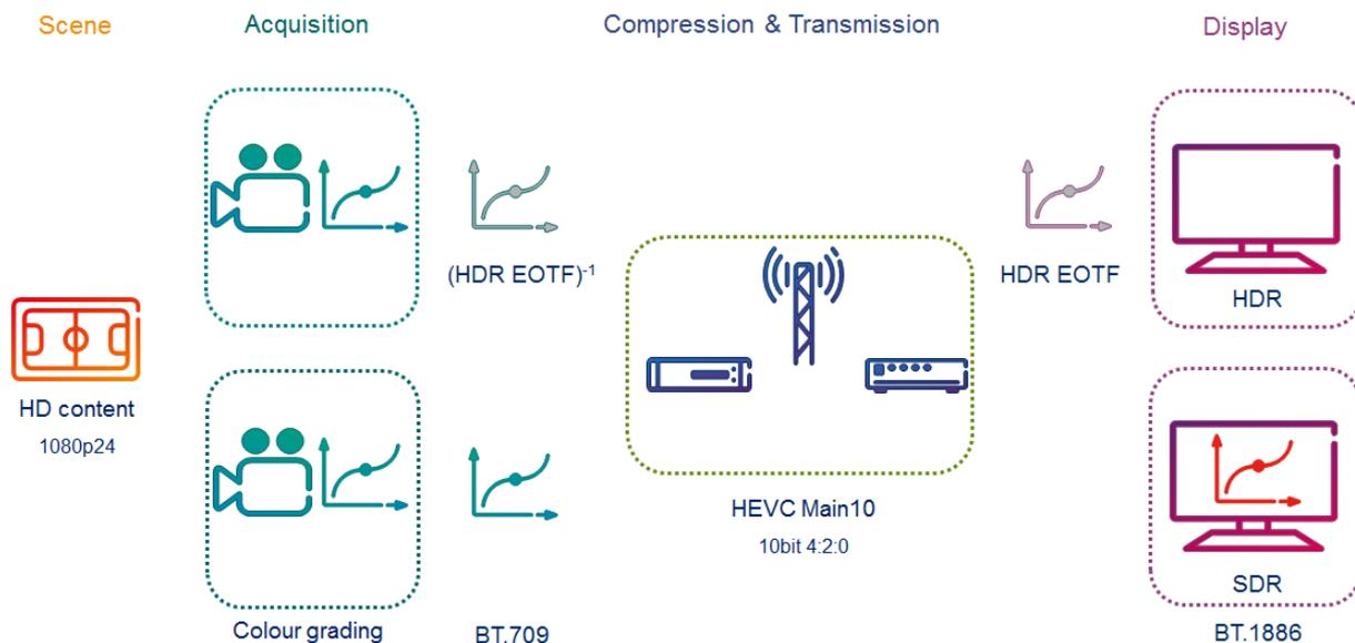
Figure 2 – Diagram of simulated HDR and SDR broadcast systems
