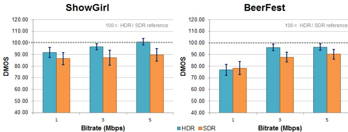
Figure 5– DMOS results for the ShowGirl (left) and the BeerFest (right) sequences. The error bars represent 95% confidence intervals
