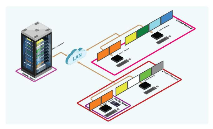
High-performance IP KVM extenders can streamline operations, control costs, and increase local and remote collaboration between operators. In this environment, the physical machines can be moved from the control rooms and relocated to a secure server room, enabling operators in adjacent control rooms to access any number of workstations or servers over IP. Switching is also a must in this environment.
