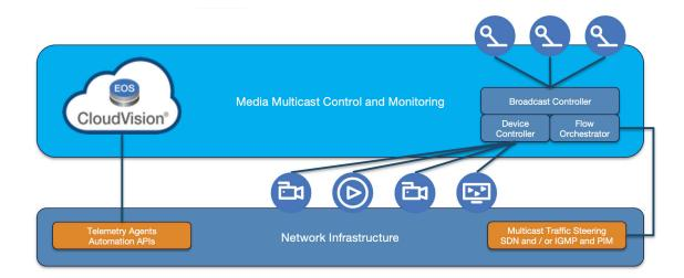
SDN (Software Defined Networking), or Flow Orchestration, is a broad term that describes the process of taking active control over exactly where the multicast flows travel in a network. To be most effective, it needs to be both bandwidth and path aware.
