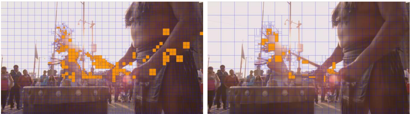
Figure 3 – Illustration of HEVC (left) and VVC (right) selected intra (in orange)/inter modes per CU.
