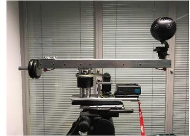
Figure 1: Motorised camera rig for background capture
