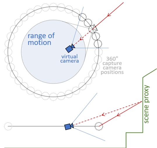
Figure 3: Top and side views of light field geometry (not to scale). Target rays (dashed red) are interpolated from source rays (solid red).
