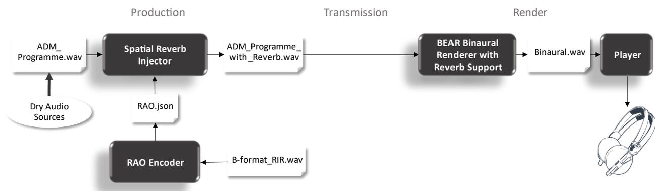
Figure 7: Room Acoustic Object processing pipeline
