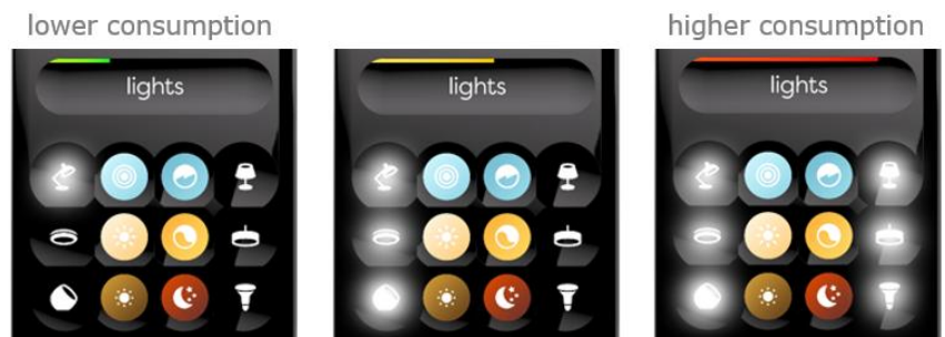
Figure 3 – remote's screen with the "consumption" gauge on top, and devices below. On the left a situation with low energy consumption, in the center more devices turned on and average consumption, and on the right, all the devices turned on and a higher consumption.
