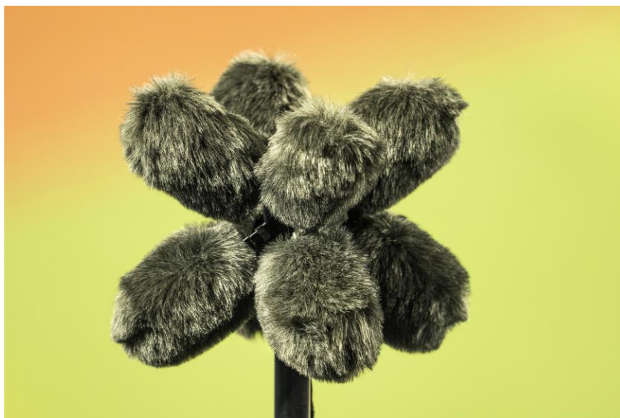
Figure 4 – An immersive 8.0 microphone was specifically designed by OBS to capture the sounds of the Olympic Games.
