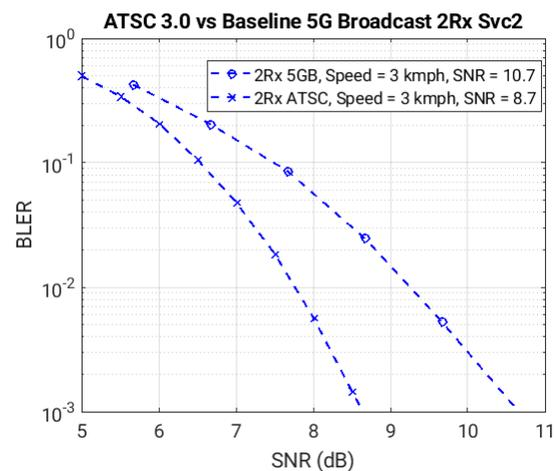
**Figure 4: Comparison over fading NLoS channels with 2Rx antennas.**
