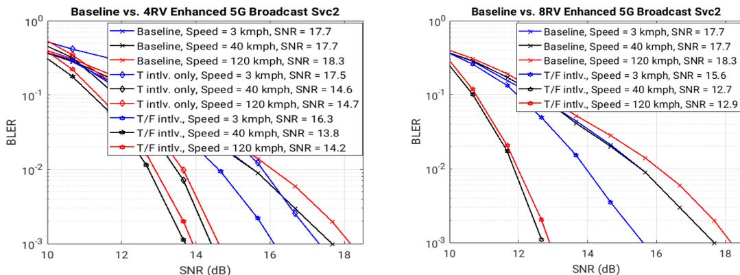
Figure 7: Performance of enhanced 5G Broadcast with proposed interleavers.
