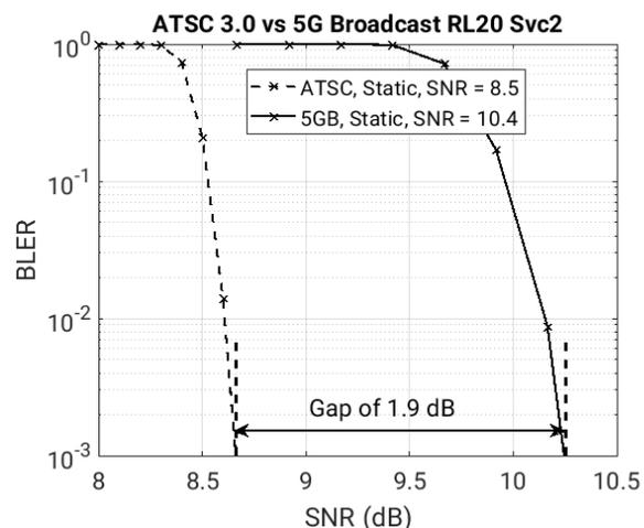
**Figure 3: Comparisons of Svc 1 and Svc 2 over the RL20 static channel.**
