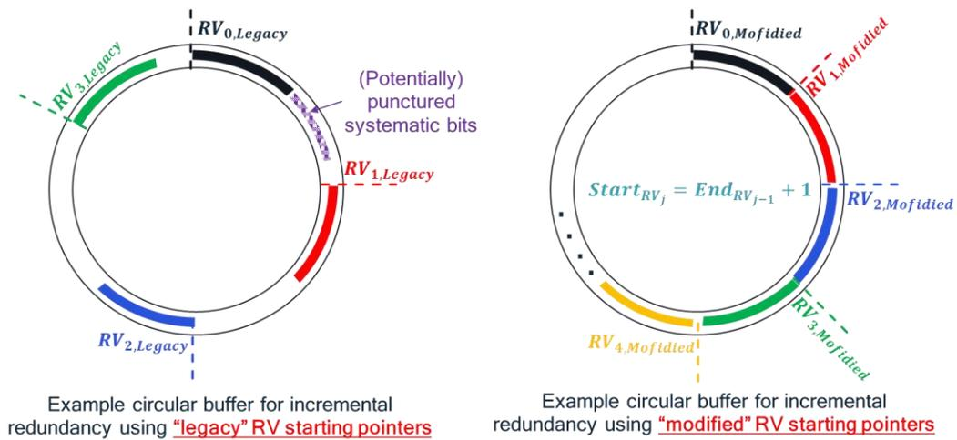
Figure 6: Illustration of "legacy" vs "continuous" RVs.
