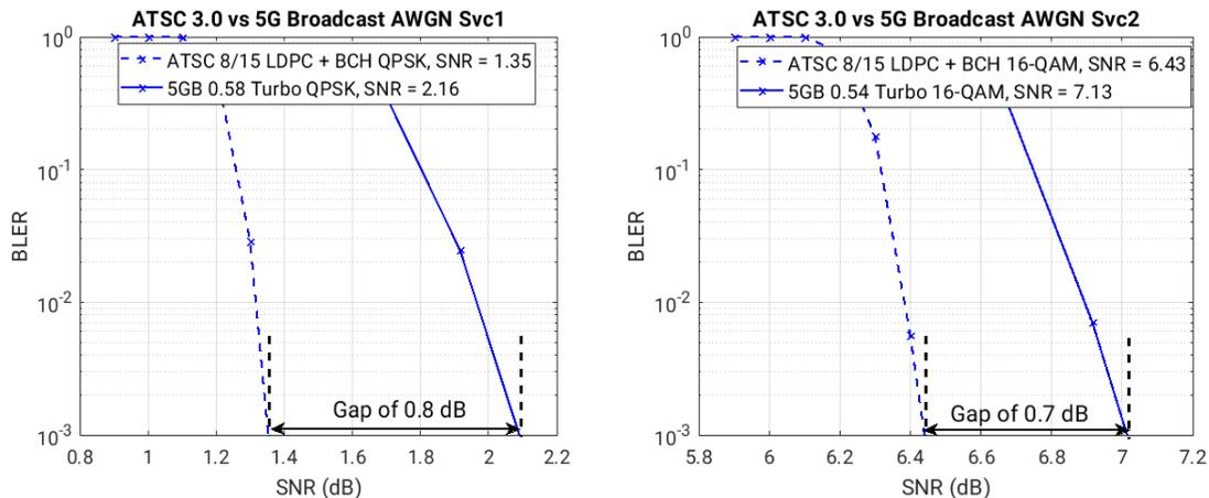
**Figure 1: Comparison for Svc 1 and Svc 2 under an AWGN channel.**
