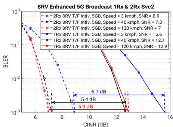
**Figure 8: Gains from 2Rx antennas.**
