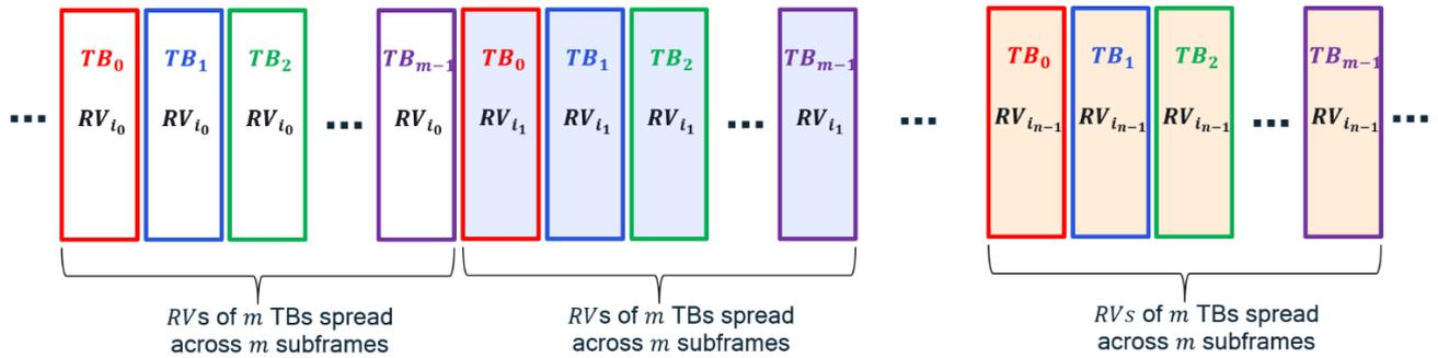
**Figure 5: Interleaved transmission of “HARQ redundancy versions” of (scaled) transport blocks across slots/subframes.**
