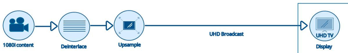
Figure 9 - Upscaling at the content provider side
