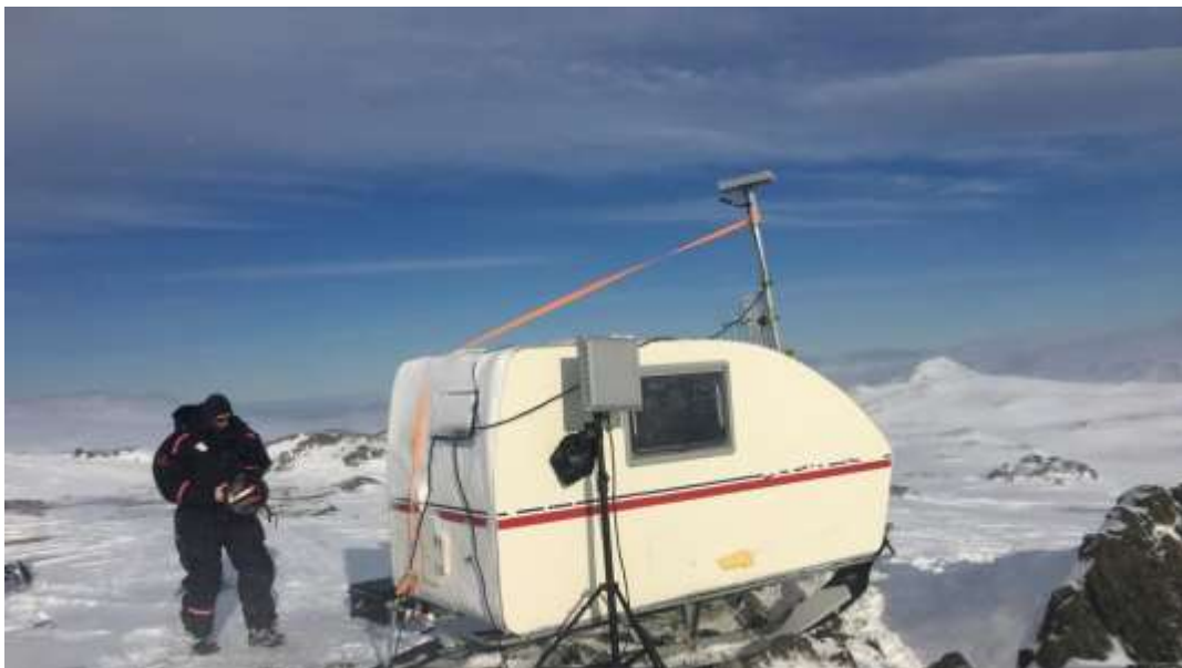
Figure 6 – One of the IP relay station sleds in position. Photo by Jon Are Kolstad.
