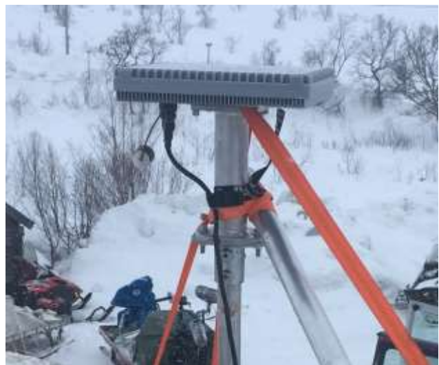
Figure 4 – Digital phased array panel mounted on top of the production sled. A single cable contains power supply and Ethernet.
