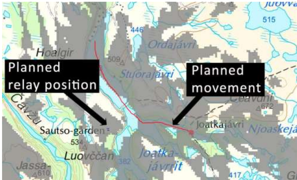
Figure 7 – Network planning on the move. Adjusting positions of the relay stations.
