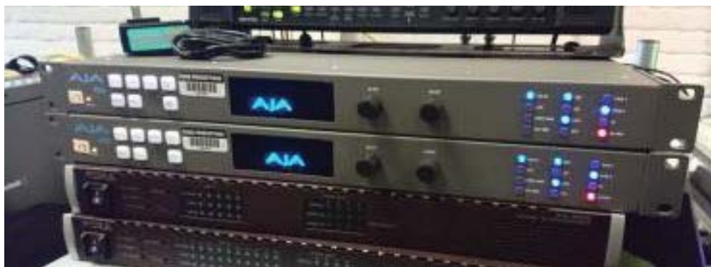
Figure 4 - The Upconverters, as used within the system.
