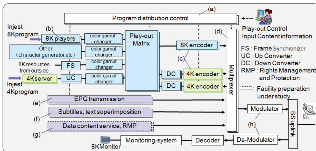
Figure 3 – Play-out / transmitting equipment for test broadcasting
