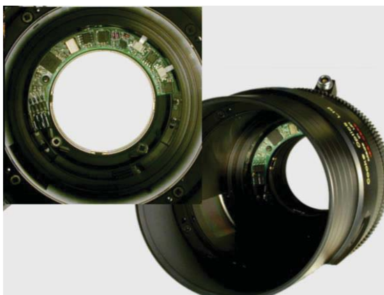
Figure 3 - Inner workings that show the i boards in a lens housing
