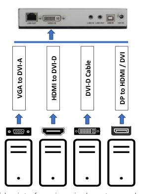
more current computers with different video interfaces in a single system and allow the swap-out of computers with different interfaces without having to procure different Tx units.
