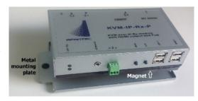
be pulled out and put back in place very easily without using tie wraps or tape.
