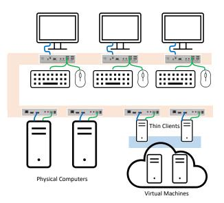
virtual machines would be to connect regular Tx to actual thin clients (see the diagram.) This requires a bit more hardware but will guarantee the proper shield between the two networks. Furthermore, the thin client consoles could be used as local back up consoles.
